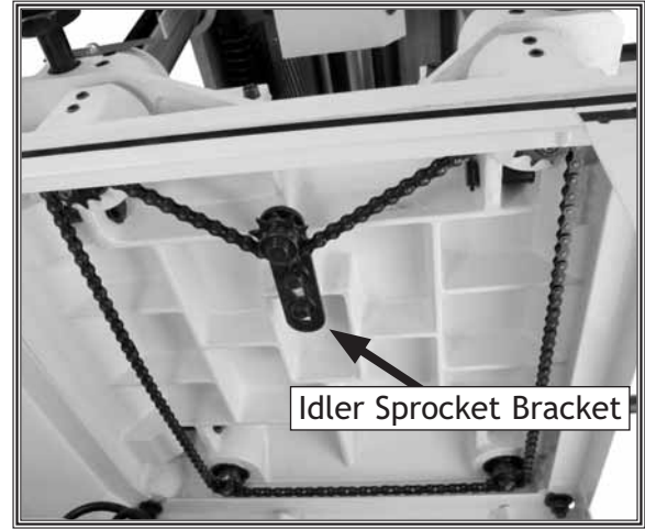
Figure 34. Chain drive system.
